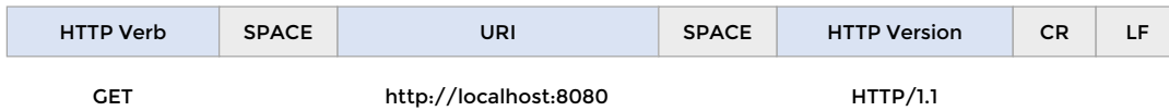
Figure 13.3: Representation of a request. Blank spaces exists between each part of the request. In the version HTTP/1.1 the request requires the CR and LF characters at the end.
